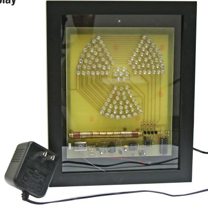
If the Radiation Illuminator Display is going to be operated from a 9V battery turn the kit off using the on/off switch and make sure the AC adapter is unplugged before connecting your 9V battery, after the battery is connected turn the switch back to the on position. The GM tube used to detect radiation uses high voltage so reversing polarity of the power source may cause damage to the components.
