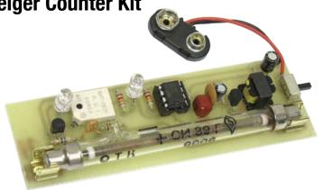
This kit should not be handled while power is supplied. The GM tube uses high voltage at very low current, so handling the kit during operation may cause shorts or component failure (the current is very weak and will not cause harm to you but can damage the components in the kit). This kit should be enclosed within a plastic case during operation. Sorry, we do not have a case available for this geiger counter kit.
