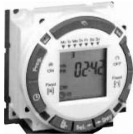
The DT20 is a compact electronic 24 hour/7 day time switch module, with heavy duty relay contacts for switching low or line voltage loads. Applicable for time of day control of pumps, fans, heaters, HVAC control circuits, lighting, machinery and many other types of commercial, industrial, and agricultural equipment.
