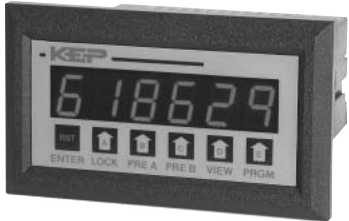
**Preset Counter:** 5 digit display with a 5 digit dividing scale factor. Two, 5 digit, programmable setpoints are available for output control. Display flashes when either output is active.
