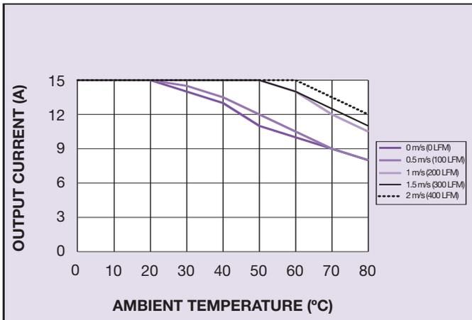
Figure 9 - Maximum Output Current vs. Ambient Temperature and Airflow for SIL15C-12SADJ with Vout set to 5 V
