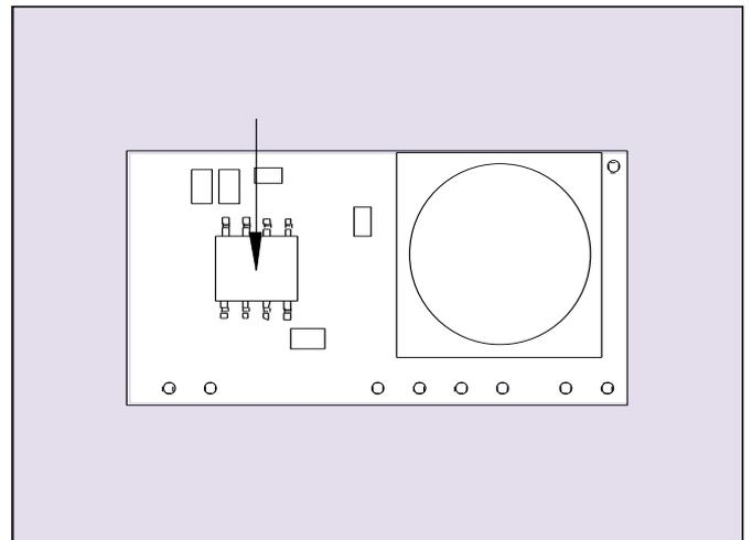
Figure 12a - Thermal Reference Point Location on SIL06C Converters
