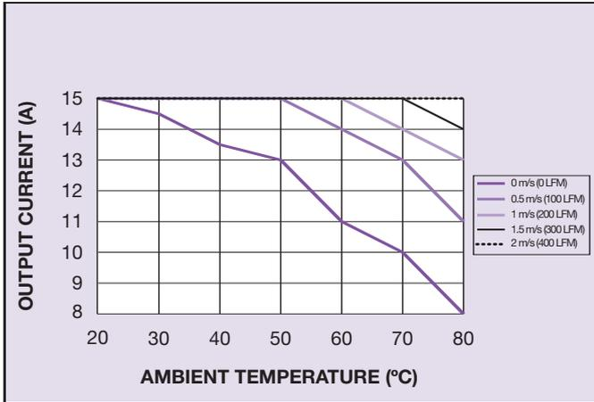
Figure 8 - Maximum Output Current vs. Ambient Temperature and Airflow for SIL15C-12SADJ with Vout set to 0.9 V
