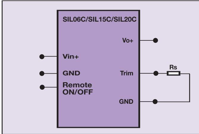
Figure 13 - Trimming Output Voltage using External Resistor
