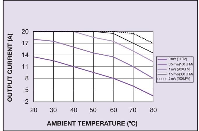
Figure 11 - Maximum Output Current vs. Ambient Temperature and Airflow for SIL20C-12SADJ with Vout set to 5 V
