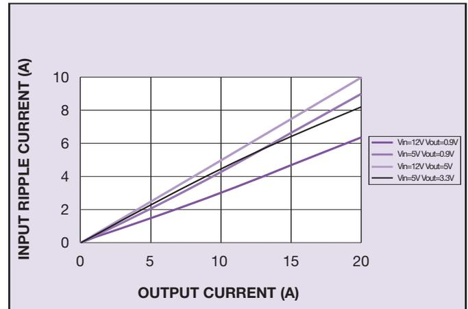
**Figure 18 - Input Ripple Current with Output Current**
