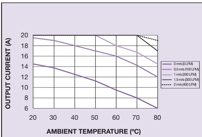
Figure 10 - Maximum Output Current vs. Ambient Temperature and Airflow for SIL20C-12SADJ with Vout set to 0.9 V
