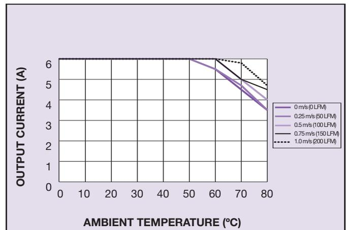
**Figure 7 - Maximum Output Current vs. Ambient Temperature and Airflow for SIL06C-12SADJ with Vout set to 5 V**
