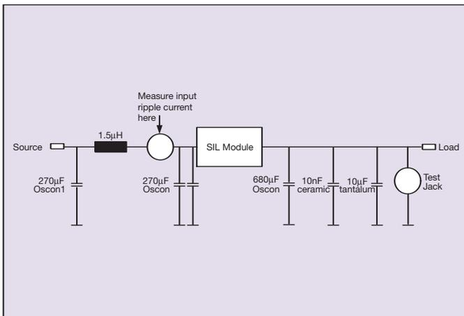
**Figure 17 - Input Reflected Ripple/Capacitor Ripple Current and Output Voltage Ripple and Noise Measurement Set-Up for SIL20C**
