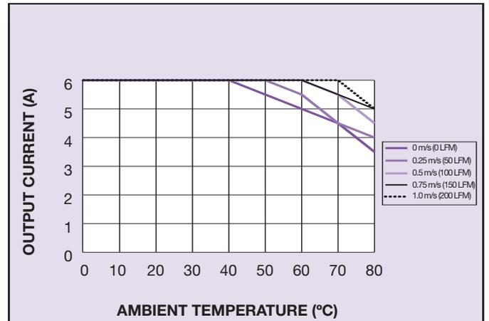
**Figure 6 - Maximum Output Current vs. Ambient Temperature and Airflow for SIL06C-12SADJ with Vout set to 0.9 V**
