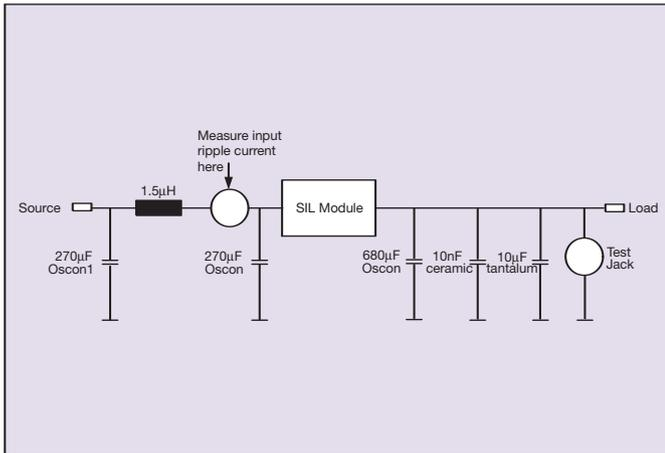
**Figure 16 - Input Reflected Ripple/Capacitor Ripple Current and Output Voltage Ripple and Noise Measurement Set-Up for SIL06C and SIL15C**
