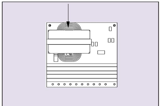
Figure 12b - Thermal Reference Point Location on SIL15C and SIL20C Converters
