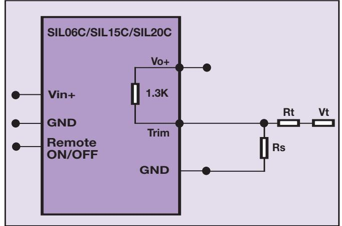
Figure 15 - Trim Output Voltage - with Voltage Source
