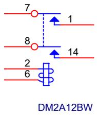
I could not find a data sheet for this specific part number but this should be accurate. It may have the diode included. If it does pin 2 must go towards +V.
