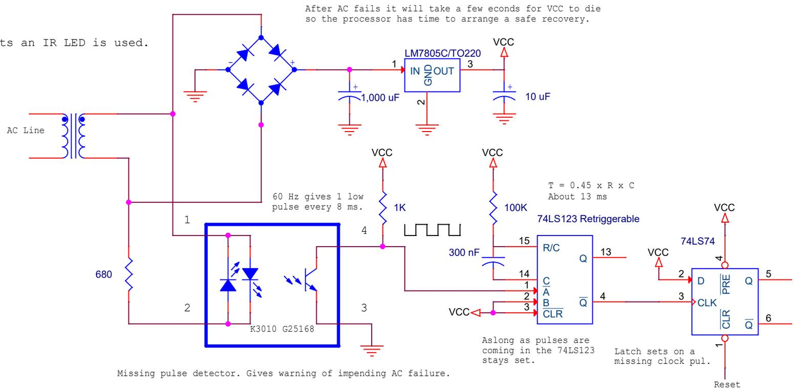
Missing pulse detector. Gives warning of impending AC failure.
