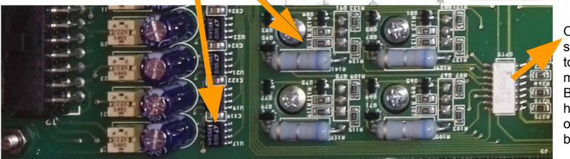
Opto coupler sends cell status to the microprocessor. Bottom off pcb has optocouplers for balancer control
